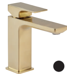
Metric basin mixer with click waste 52(w) x 160(h) x 160mm(d) Minimum operating pressure 0.2bar
