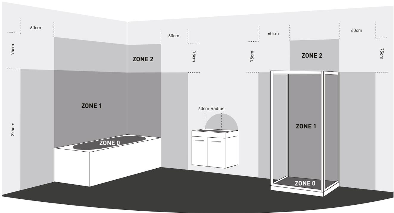
It is important to install light fittings and electric Towel Warmer elements in the correct bathroom zone i.e. the zone referred to in the IP rating of the element. This is not an installation guide and reference should be made to the latest edition of the IET Wiring Regulations or a qualified electrician member of NICEIC or IET.
