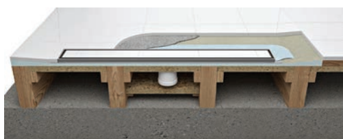
Tray & Drain using underboarding, including under trap
